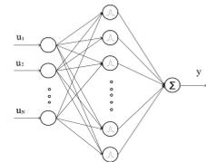
The structure of Radial Basis Function Neural Networks.
